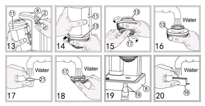
13. Fig 13 Grasp the main body tightly, press the press button, and take out the main body by leaning outward. Before pressing the press button, make sure the main body is gasped tightly, otherwise the main body will fall down.
